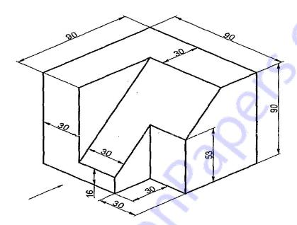
Q9) Figure show orthographic views of an object by first angle method of projection. Draw its isometric view. [16]
