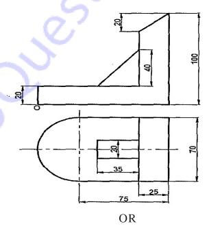
Q10) Figure show orthographic views of an object by first angle method of projection. Draw its isometric view. [16]
