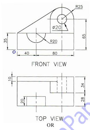
Q8) Figure shows front view and right hand side view of an object. Draw Isometric view and show overall dimensions.[12]
